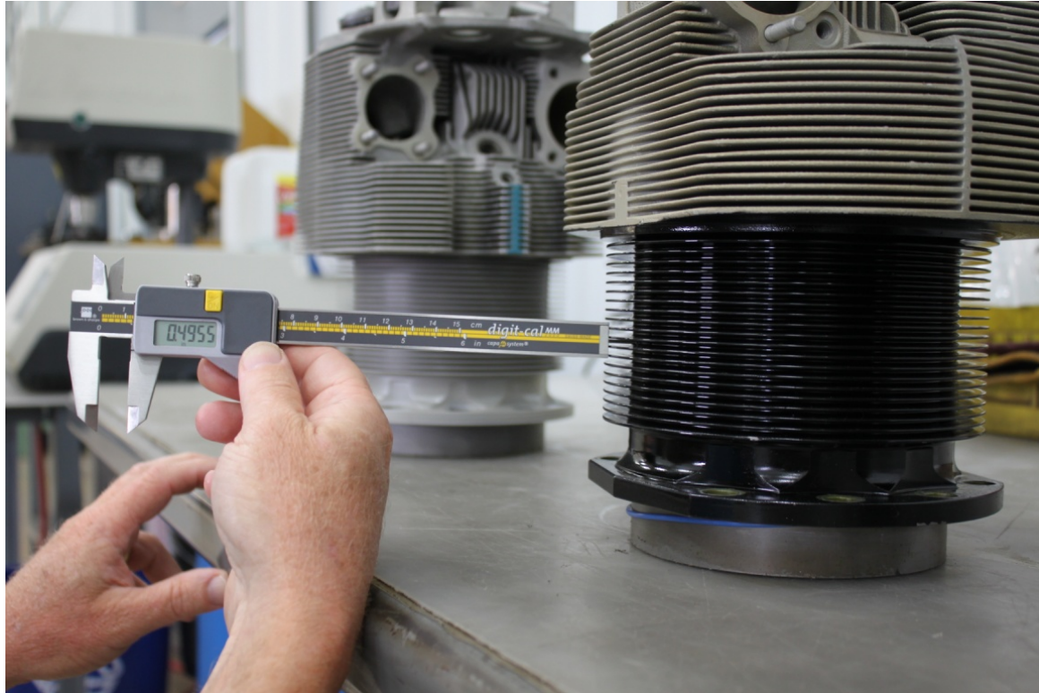
Photograph 1 Measuring Fin Depth Using A Caliper
