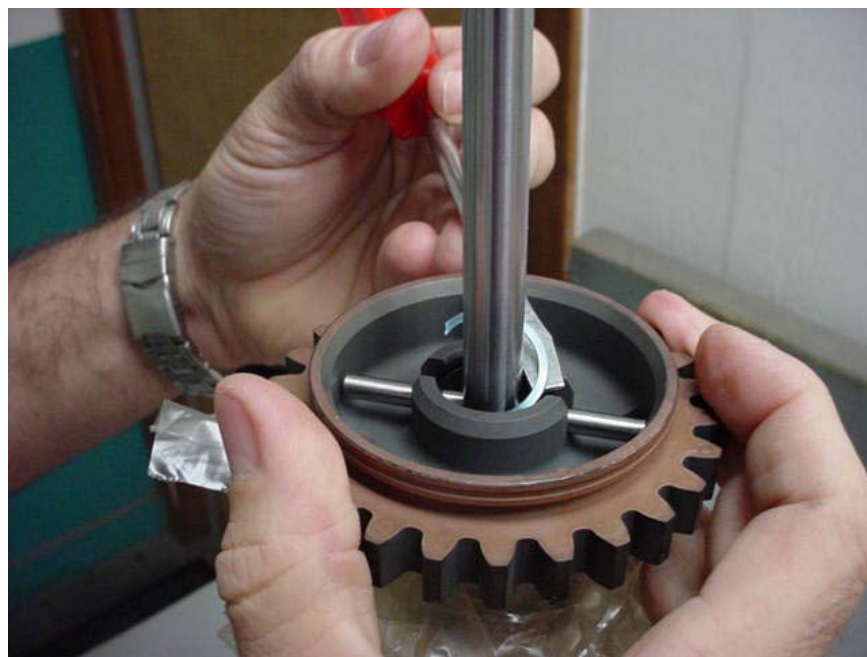
Figure 2: Disassembly of the Spiral Retaining Ring
