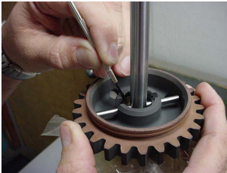
Figure 1: Picking the End of the Ring Out of the Groove
